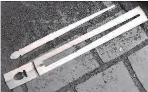
The cardboard template. It folds in half to check the contours against the wood.
