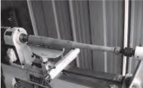
Roughing the wood. The dreaded dowel is visible in the middle of the wood.
